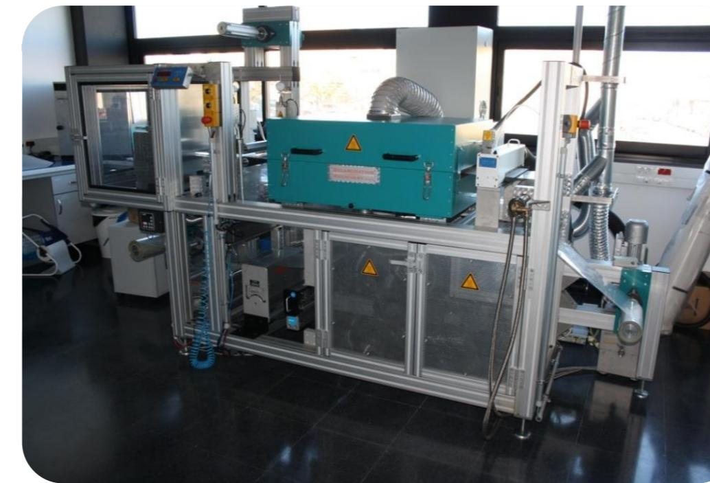
Roll to Roll Slot-die and foulard coating and lamination
