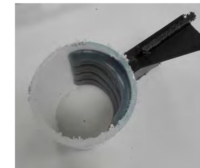
Junction detail: In white the blown tube, in black injected part
